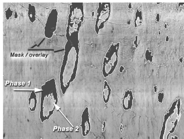
Fig. 8. Image analysis on PP-2. The contrast between the matrix, the EPR part of the segregated phases as well as the crystalline inclusions in the segregated phases is enhanced and masks are defined.
